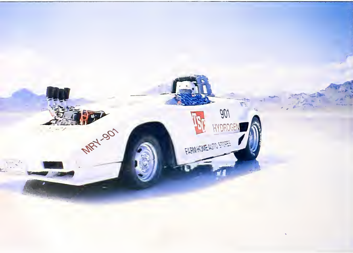
This hydrogen-powered Lamborghini replica (shown at the 1992 Bonneville Speed Week, Wendover, Utah) has a 1990 Nissan engine stripped of all electronics and pollution controls.
