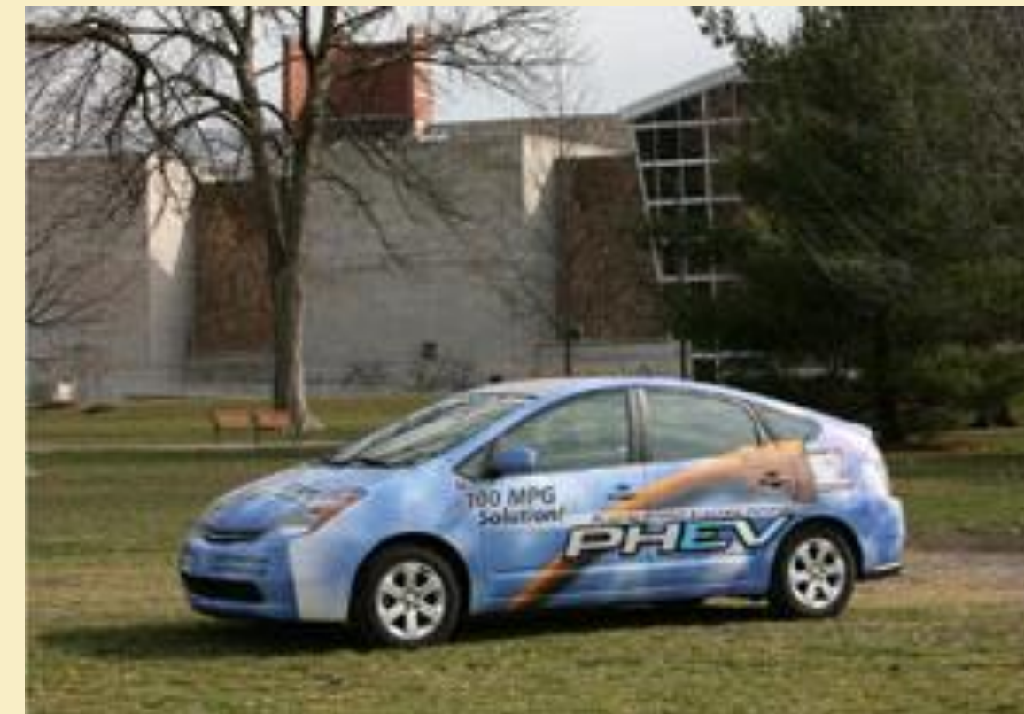
Fig 1: Toyota Prius converted into PHEV
