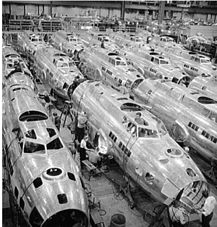
Production of B-17 F (Flying Fortress) fuselage sections. Library of Congress, Black-and-White Photographs from the FSA-OWI, 1935-1945 (LC-USW3-041070-E).
