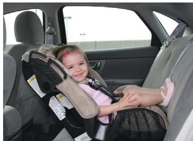
An 18 month old child properly positioned in a rear-facing convertible child safety seat.
