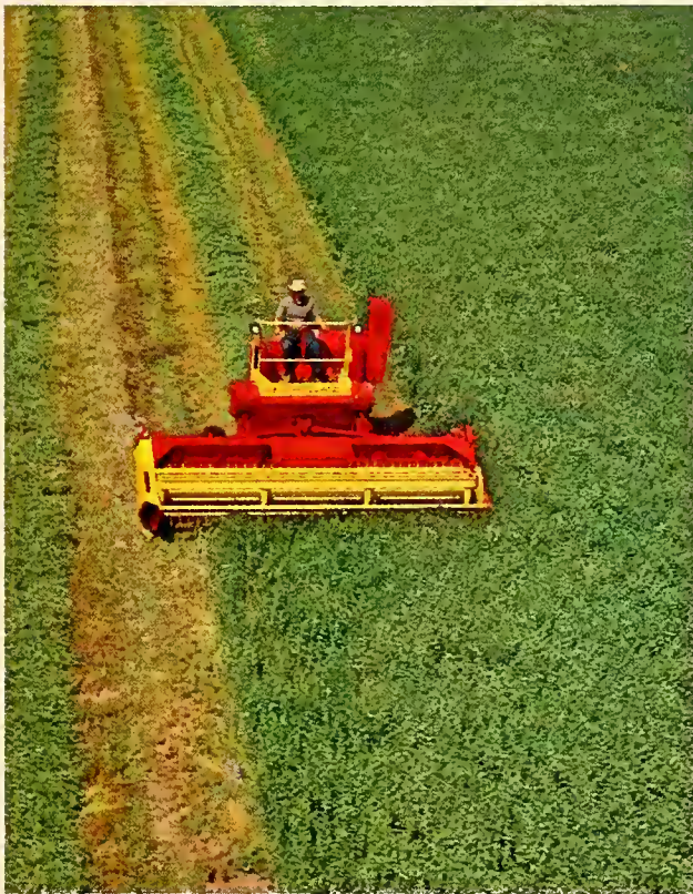
Model 909 Speedrower® self-propelled windrower is available with 12-, 14-, and 16-foot auger headers.
